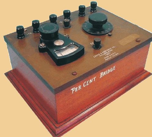
Figure 1. Balanced bridge with voltmeter as null detector.
